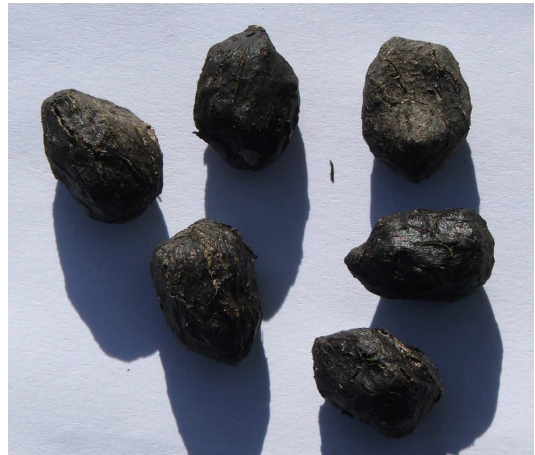
Non-degraded pellets, although cracked, no loss of material has occurred
